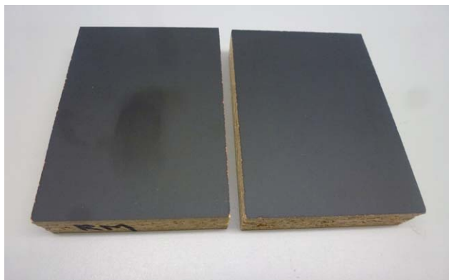
Figure 9. Fingerprint application and removal after 10 double-rubs Left: Matt LPM laminate with standard resin; Right: Matt LPM laminate with PDMS-CHO. [Color figure can be viewed in the online issue, which is available at wileyonlinelibrary.com .]
